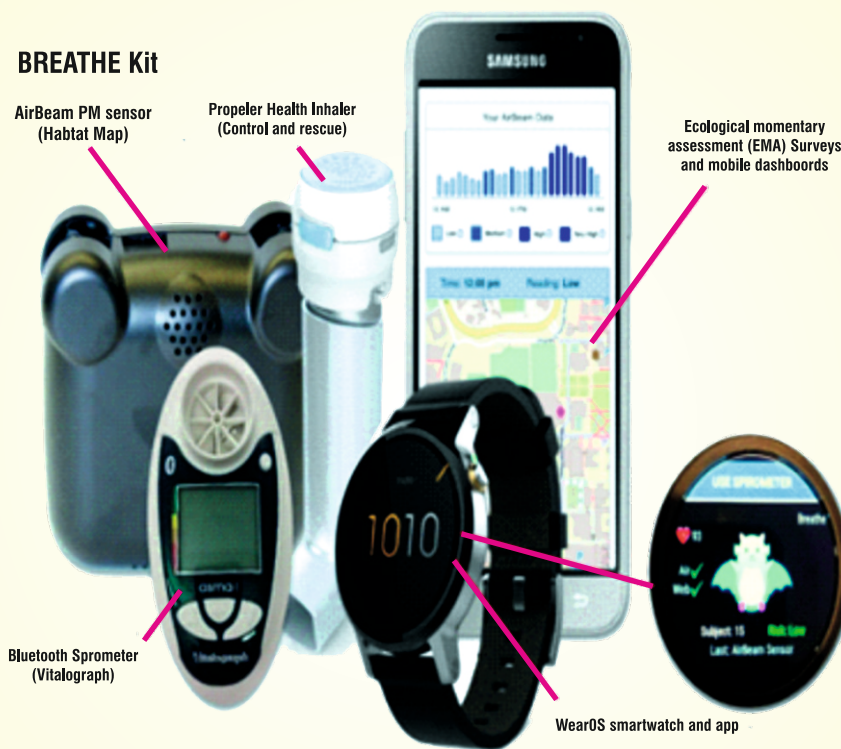
Some of the Personal monitoring devices and geospatial technologies which were useful in understanding the effect of personal environmental exposures.
